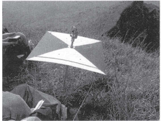
(b) Marker installed on site for use as reference point in digital photogrammetric analysis
