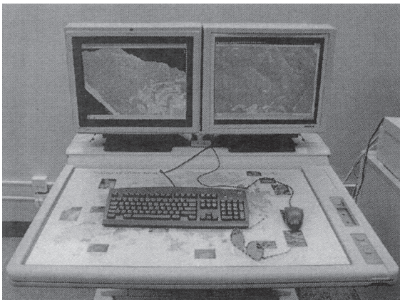
Figure 2. Digital photogrammetry workstation (Note: stereo view displayed on computer monitors)
