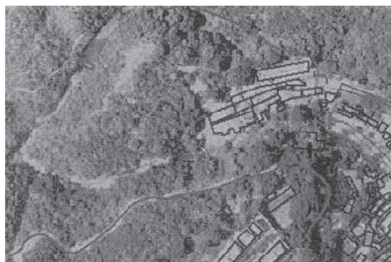
(b) Ortho-rectified image (Note: true to scale and position-accurate)
